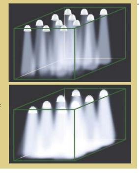
Not all lighting fixtures are created equal. Inferior optic design can actually require more fixtures and provide less uniform illumination (top). Optimized optical control can dramatically improve distribution and uniformity, with fewer lighting fixtures (bottom). Photos: Holophane
